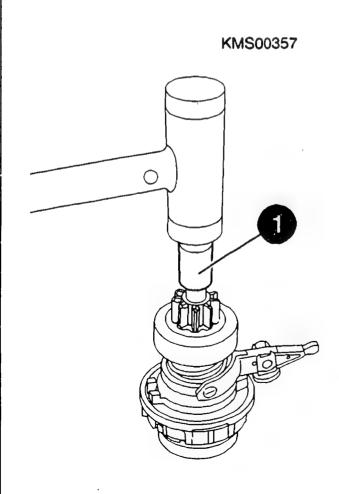
Disassembling overrunning-clutch drive
